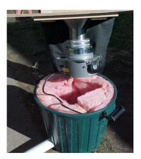
The pump draws air through a fiber filter. The insulation muffles the noise.
