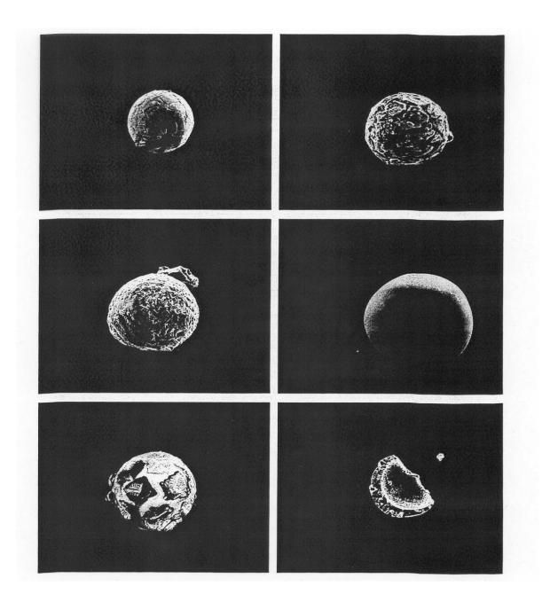
Figure 1: Scanning electron microscope photographs of five magnetic spherules and one spherule fragment. Diameters range from 15 to  $20\mu m$ . The photograph of the fragment shows that larger spherules may contain cavities.
